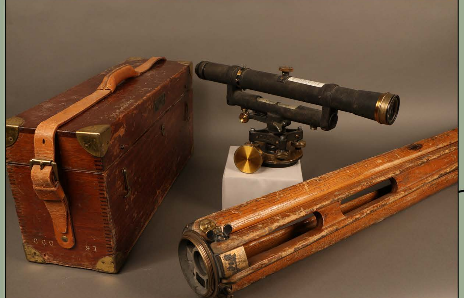
Catalog # 1999-011-002 Brass transit scope with wooden tripod used by CCC Camp BR-91, in Pleasant Grove. This camp was involved with building of the Deer Creek Dam.
